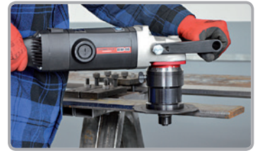
Steel plate beveling
