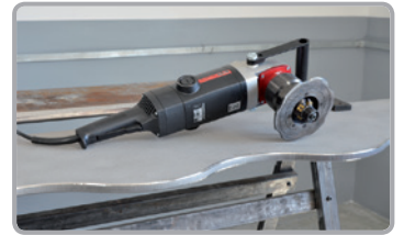
Arched edge beveling with radius
